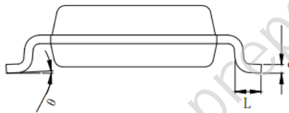
Figure 23. SOP-8 Side View
