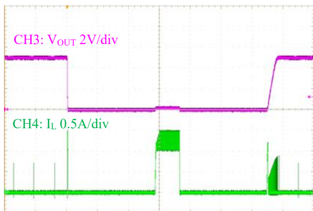
V_{IN}=48V I_{OUT}=0A Time(10ms/div) Figure10. Short Protection and Recovery
